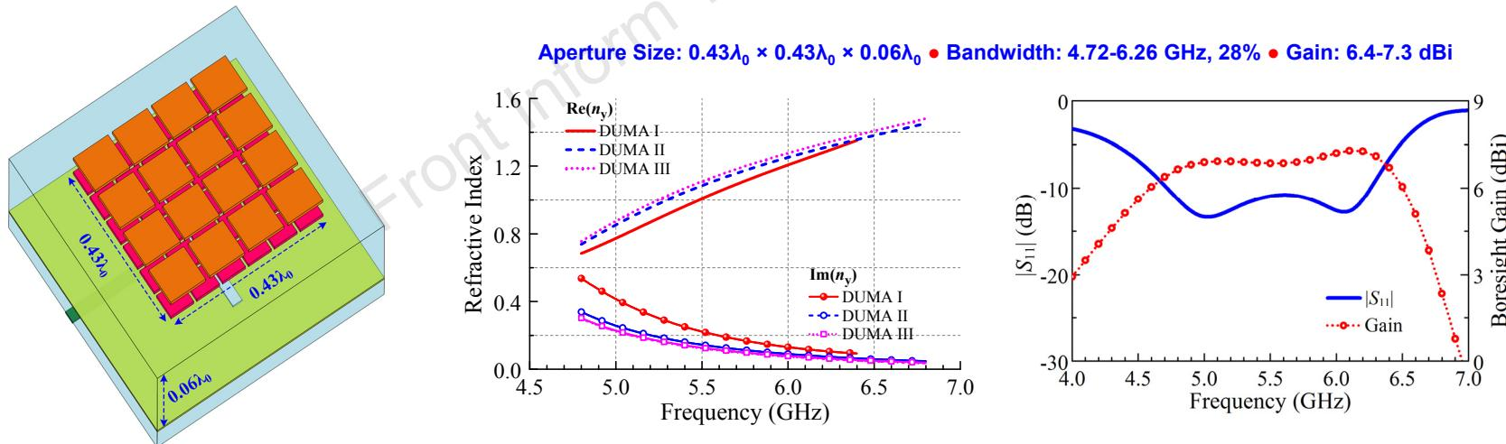
Further enhance capacitive coupling with dual-layer metasurface
