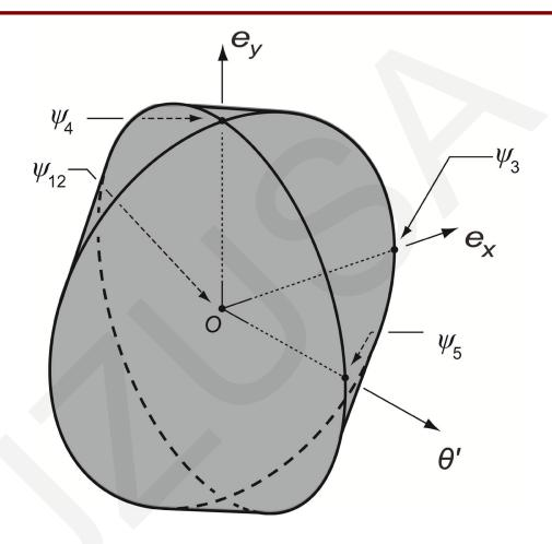
T-Map of Fig. 8 for the MSP of the arc-slot in Fig. 1a, now transformed to the canonical global *Pxy*-frame. Both circular edges have diameter *t*
