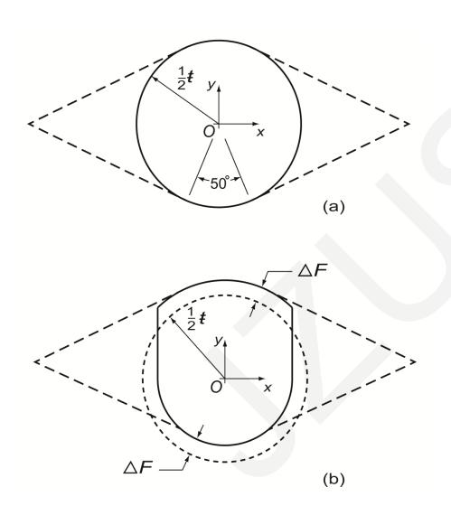
2D T-Map primitives for the arc-segments of the curved slot in Figs. 1a and the dashed lines (rounded rhombus) for both arcs centered at O and the solid lines for the two arcs at R and S; (a) For the MSP; (b) For arcs 1, 2, and 4 of an arc-slot larger than the MSP by  $\Delta F$
