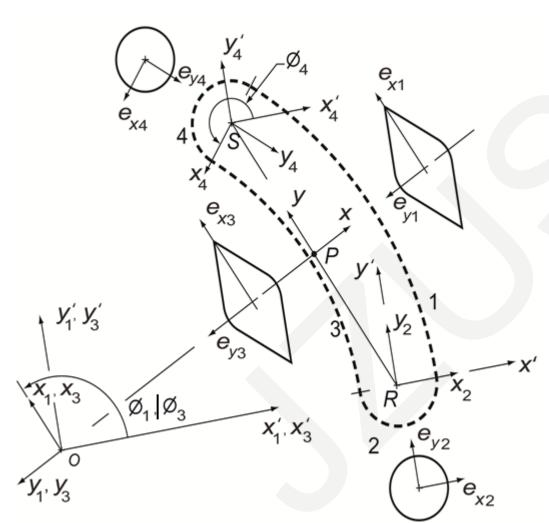
Global Rx'y'- and Pxyframes for the arc-slot in Fig. 1a which has been decomposed into four arcsegments, each with its local reference frames  $x_i y_i$ and  $x'_i y'_i$  and its 2D T-Map primitive. The angles  $\phi_i$ shown are for global frame Rx'y'
