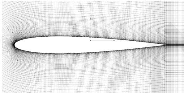
Fig.4 local grid distributions around NACA 0012.
