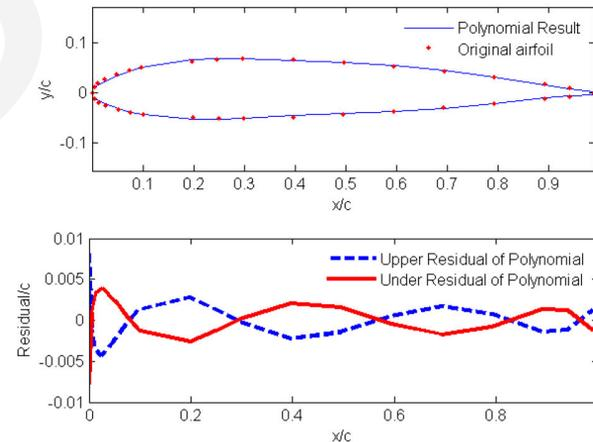
Fig. 2 Comparison between NACA 1412 airfoil and the fifth-order **Polynomial** imitation result.
