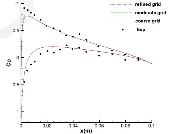
Fig.5 Wall pressure coefficient comparison of NACA 0012.
