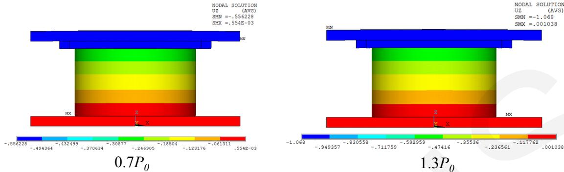
Fig.6 Vertical displacement of the SLRB model (mm)
