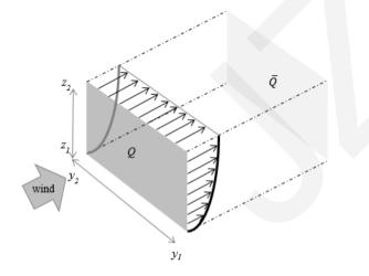
The equivalent air flow for a control domain (Q) within a larger computational domain, whose boundary condition for the inlet is defined by a logarithmic wind velocity profile, can be obtained by its perpendicular projection (surface y-z).
