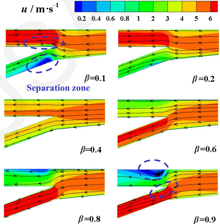
Flow structure of tunnel bifurcation at different  $\beta$  ( $\theta = 10^\circ$ )
