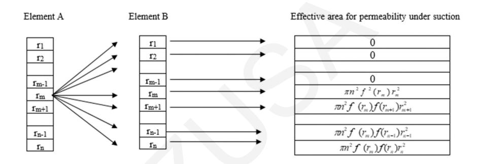
Divide the pores in soil into several groups, each group can be represented by a tube with a particular radius, r, and its statistical distribution, f(r). Consider these tubes with different radii are randomly connected on one section, then the effective area which allows water flow through the section can be calculated and illustrated in the table.
