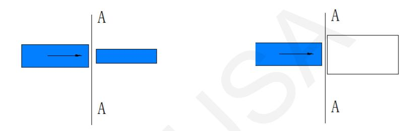
If the pores on the both sides of section A are wet, then the water can flow through section A. If the water in the big pore on the one side of section A is drained out due to the applied suction, then the water cannot flow through section A because the water flow is blocked by air-water interface.
