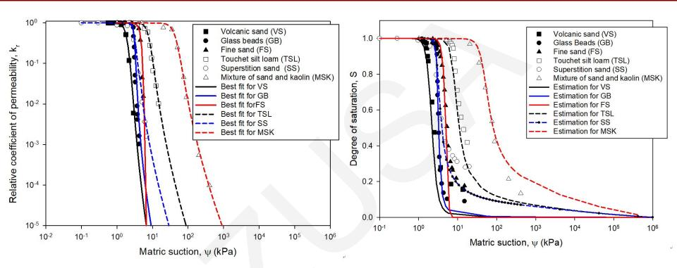
Measured data of permeability and best-fit curve using proposed equation
