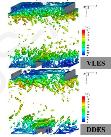
With the same mesh, the time-averaged velocity and the fluctuating velocity in the rotating state obtained by the VLES method are better predicted.
