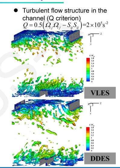
With the same mesh, the velocity distribution obtained by the VLES method in a static state has higher accuracy, and it captures more wall turbulence structures
