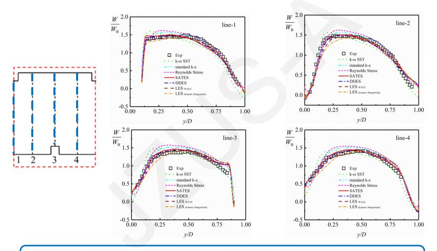
With the same grid, compared with the simulation results of other methods, the VLES method is closer to the experimental data.
