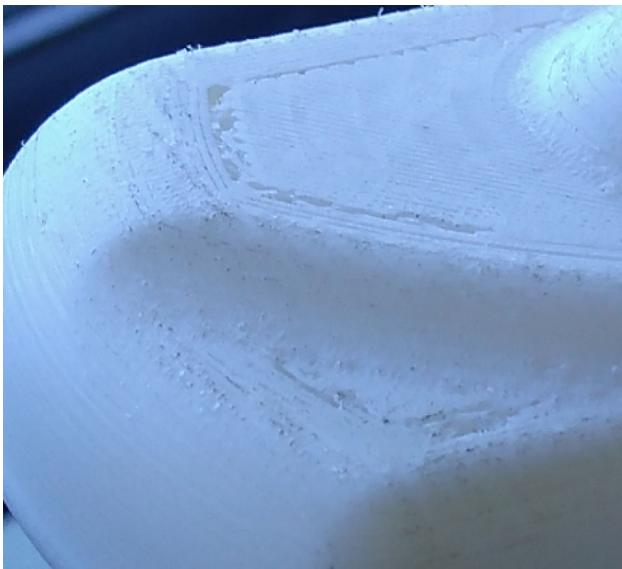
Fig. 10 Defects caused potentially by a poor adhesion between filaments
