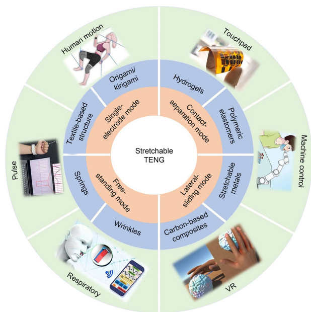
Fig. 1 Illustration of the demands of stretchable TENG for wearable bioelectronic devices. Image for “Human motion” was reproduced from Ref. [35], Copyright 2022, with permission from the American Chemical Society. Image for “Pulse” was reproduced from Ref. [36], Copyright 2023, with permission from the authors, licensed under CC BY 4.0. Image for “Respiratory” was reproduced from Ref. [37], Copyright 2022, with permission from the authors, licensed under CC BY-NC-ND. Image for “Touchpad” was reproduced from Ref. [38], Copyright 2020, with permission from Elsevier. Image for “Machine control” was reproduced from Ref. [39], Copyright 2022, with permission from Wiley-VCH GmbH. Image for “VR” was reproduced from Ref. [40], Copyright 2022, with permission from the authors, licensed under CC BY 4.0. TENG: triboelectric nanogenerator; VR: virtual reality
