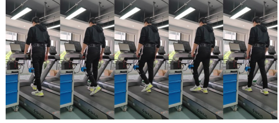
Fig. 9 Experiments on wearing the knee exoskeleton on the treadmill
