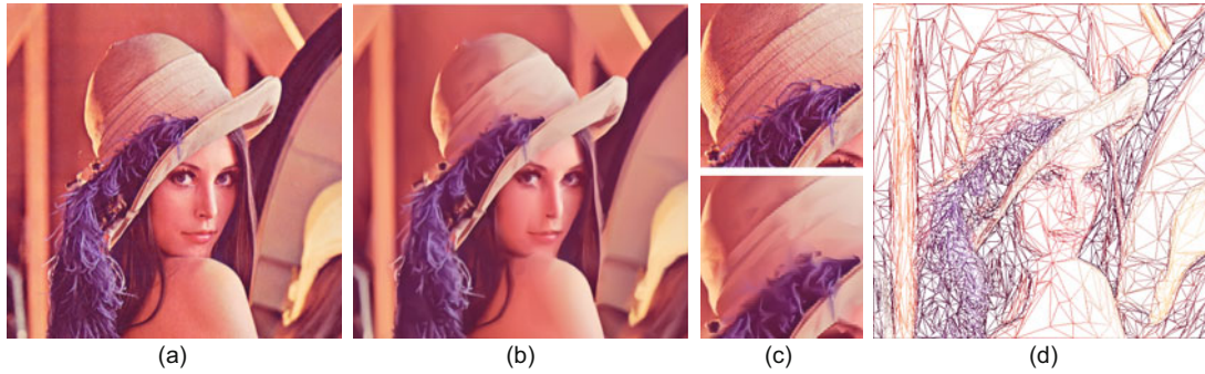
Fig. 1 Inputs and outputs. Given an image, ‘Lena’ (a), and the sampling ratio (1% in this example), our algorithm generates a mesh-based vector graphic (d) with its rendered result (b). Detail regions of both (a) and (b) are enlarged and shown in (c), in which upper and lower parts correspond to (a) and (b), respectively. References to color refer to the online version of this figure
