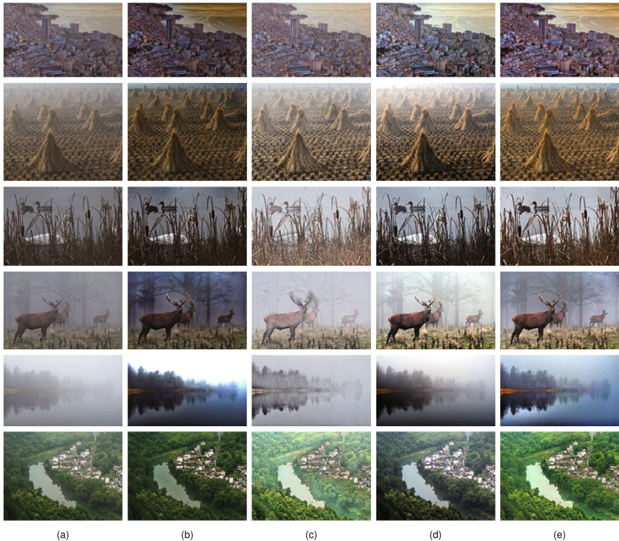
Fig. 12 Comparison on foggy images: (a) input image; (b) dark channel prior; (c) bright channel prior; (d) linear histogram stretching globally; (e) double channels with adaptive patches
