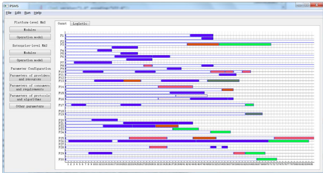
Fig. 12 User interface of the developed software prototype system for multi-agent scheduling in a platform-based smart manufacturing system (PSMS)
