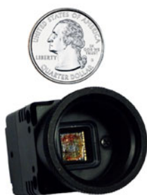
Fig. 14 A quantum dot micro-spectrometer in the form of a digital camera with electronics and circuits
