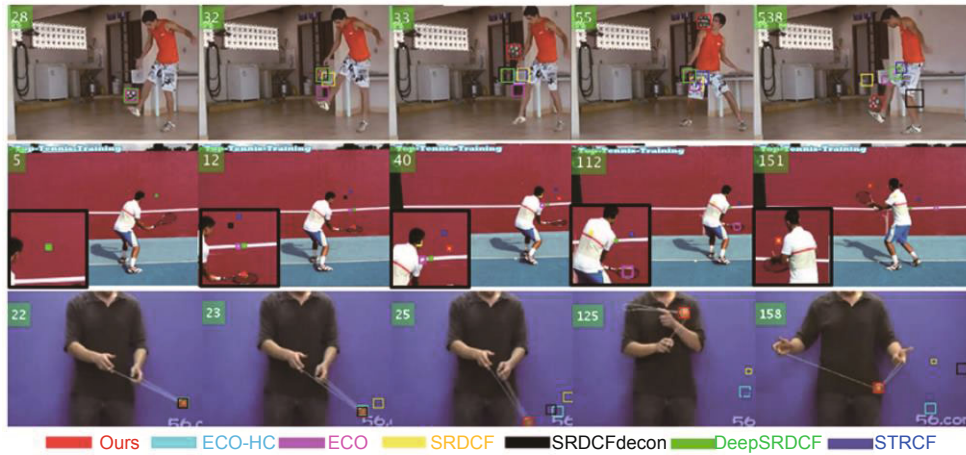
Fig. 1 Qualitative comparison of our approach with state-of-the-art trackers on two sequences with large translations of objects. Note that all the competing trackers fail on the sequences
