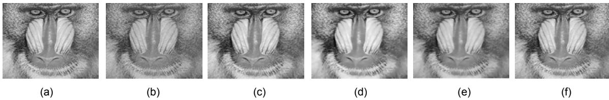
Fig. 5 Comparison results of the mandrill image: (a) original image; (b) noisy image; (c) results of the Gauss filter; (d) results of the ROF model; (e) results of the PM model; (f) results of our TVF model
