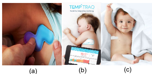
Fig. 3 Example of plaster-type thermometers: (a) Fever Scout device, manufactured by VivaLNK Co. (VivaLNK, 2020); (b) TempTraq thermometer, manufactured by Blue Spark Technologies, Inc. (TempTraq, 2021); (c) Tucky wearable thermometer, produced by E-takescare Co. (E-takescare, 2021)
