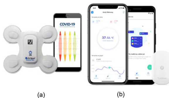
Fig. 6 Smart patch developed by LifeSignals Co. for monitoring patients' main vital signs (a) and a wearable thermometer "Celsius" produced by the Smartr Health company, placed in the armpit, to remotely monitor the user's temperature (b) (Celsius, 2020)
