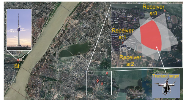
Fig. 10 Geometry of one transmitter, three receivers, and the area of interest
