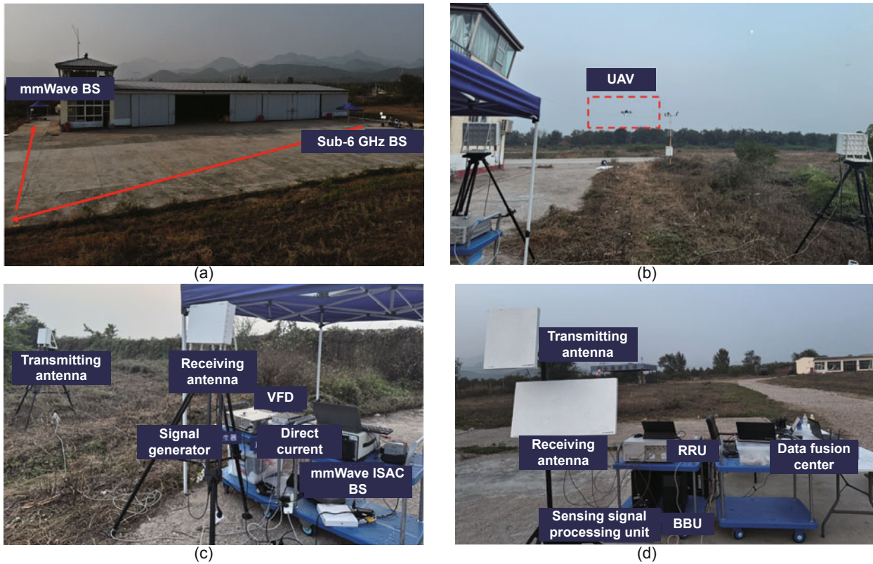
Fig. 7 Field test for multi-frequency collaborative ISAC in low-altitude UAV detection: (a) diagram of the field setup; (b) UAV with RCS \leq 0.1 \text{ m}^2 ; (c) field test scenario for the mmWave BS; (d) field test scenario for 3.75 GHz BS. VFD: variable frequency drive; RRU: remote radio unit; BBU: baseband unit. References to color refer to the online version of this figure
