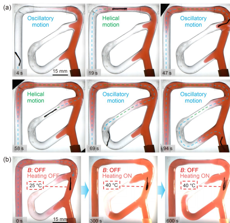
Fig. 4 Locomotion and drug delivery of microrobots in the model. (a) The mode-switchable microrobot (MSM) traverses the vascular model by employing a dual-mode locomotion mechanism. (b) The MSM achieves drug release upon near-infrared irradiation, heating to 40 °C in a vascular model
