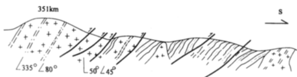
Fig. 5 Ductile deformation near the 351km road sign area
