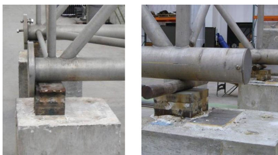
Fig. 2 Boundary condition of experimental setup
