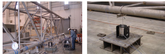
Fig. 3 Experimental setup of the Electro-dynamic shaker
