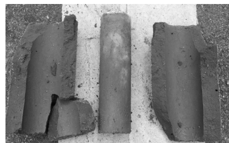
Fig. 7 Failure surface of the shear test
