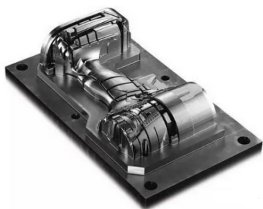
Fig. 13 A hybrid manufacturing process mold developed by the Japanese Matsuura Machinery Corporation
