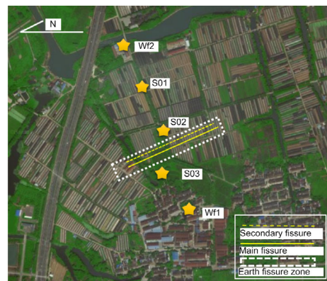
Fig. 10 Location of earth fissures according to the geological survey
