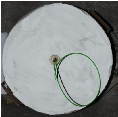
Fig. 19 UHTCC target for the blast test
