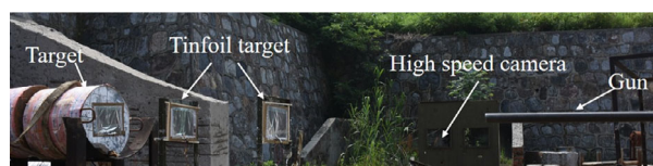
Fig. 24 Device used in penetration experiments
