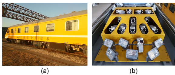
Fig. 8 Test environment: (a) catenary inspection vehicle; (b) vehicle-mounted image acquisition system
