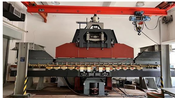
Fig. 3 High-speed maglev vehicle-rail magnetic coupling experiment platform
