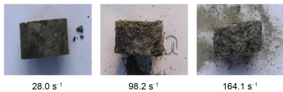
Fig. 10 Failure patterns of A-SIFCON specimens at various strain rates
