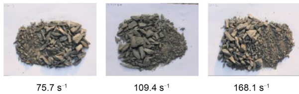
Fig. 9 Failure patterns of brittle matrix specimens at various strain rates
