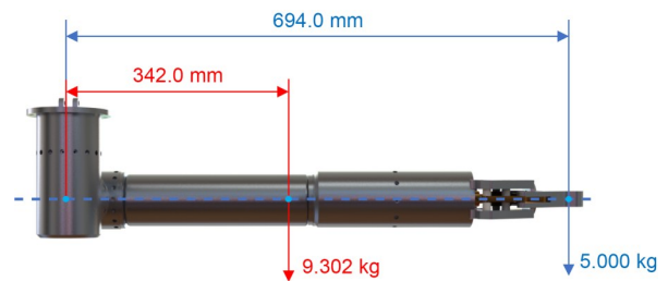
Fig. 3 Force analysis diagram of upper arm joint
