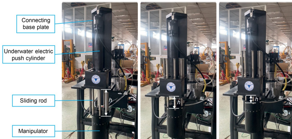
Fig. 11 Display of the working process of the lifting mechanism
