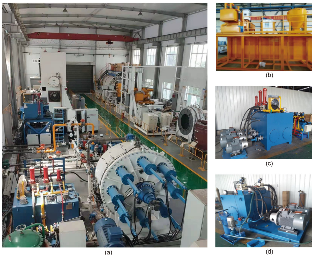
Fig. 6 \Phi 2.5 m multi-purpose test rig for slurry shield machine: (a) overview of the test rig; (b) slurry processing; (c) hydraulic system for loading; (d) hydraulic system for driving
