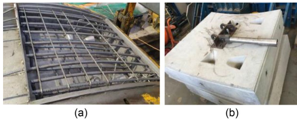
Fig. 2 Segment details: (a) steel mold and reinforcement; (b) segment
