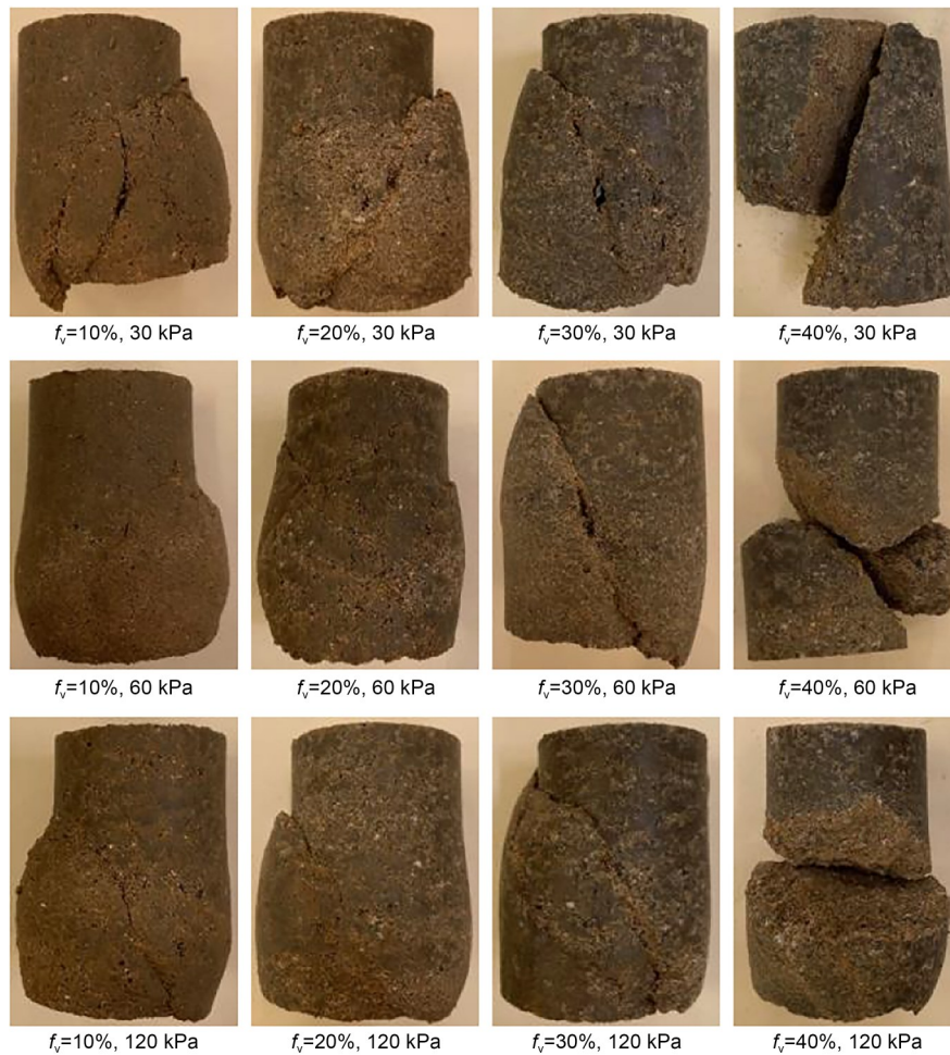
Fig. 6 Visual views of samples after shearing with D_c=95\% . The stresses in this figure represent the confining pressures
