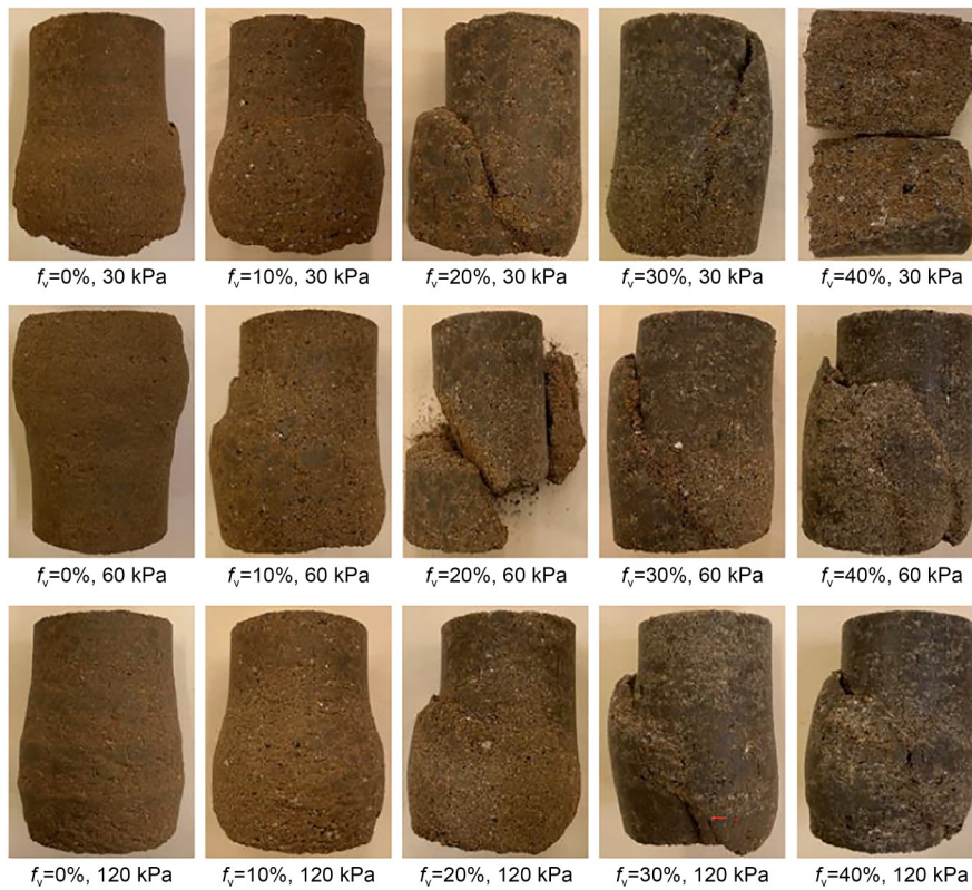
Fig. 5 Visual views of samples after shearing with D_c=90\% . The stresses in this figure represent the confining pressures
