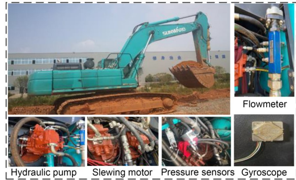
Fig. 4 The 50-t hydraulic excavator prototype
