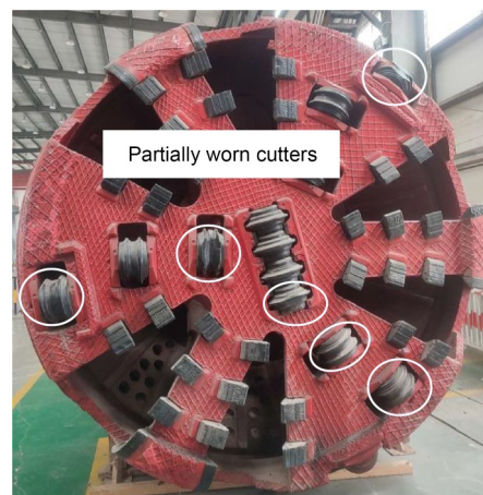
Fig. 2 Partially worn cutters in cutterhead
