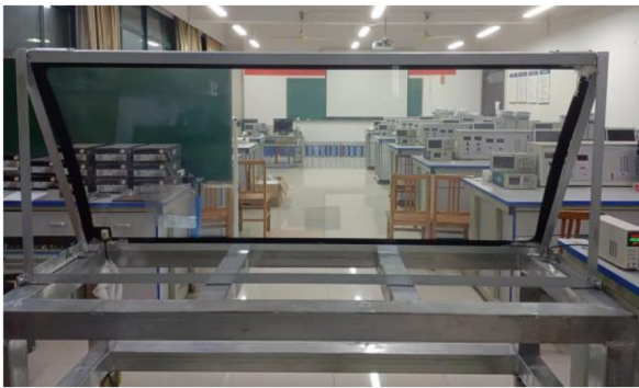
Fig. 15 Diagram of the heavy-haul locomotive windshield experiment platform
