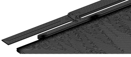
Fig. 4 Mesh refinement in corners and areas of complex flow
