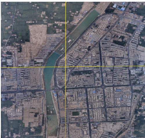
Fig. 13 Initial seam-lines generated by the Voronoi diagram (Dunhuang, China)
