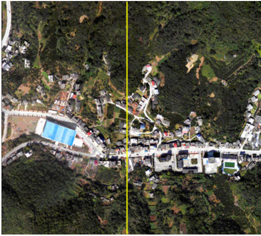
Fig. 21 Initial seam-line in a complex terrain condition (Changyang, China)
