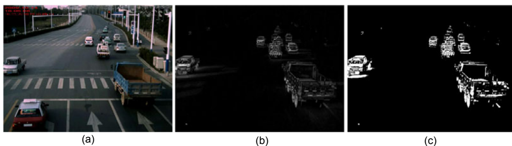
Fig. 1 Moving target detection in the video with orthogonal Gaussian-Hermite moments (OGHM): (a) middle frame of the consecutive frames; (b) middle image by OGHM; (c) binary image by the Otsu algorithm
