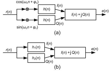
**Fig. 1** Block diagrams of conventional quadrature demodulation (a) and the proposed demodulation (b).  $h(n)$  is the impulse response of the low-pass filter and  $h_1(n)$  and  $h_2(n)$  are the impulse responses of the proposed filters
