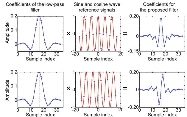
**Fig. 2 Diagrammatic explanation of designing the proposed demodulation filters ( $M = 32$ ). Top rule: derivation of the filter  $h_1(n)$  (even symmetric, for the in-phase component); bottom rule: derivation of the filter  $h_2(n)$  (odd symmetric, for the quadrature component)**
