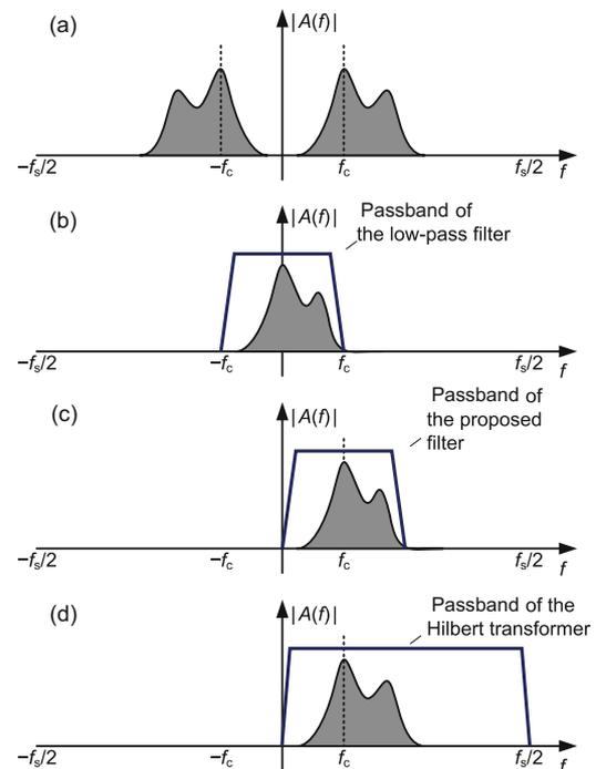
**Fig. 8** Comparisons of the proposed method and conventional methods in the frequency domain: (a) spectrum of the radio-frequency (RF) signal; (b) spectrum of the base-band signal after conventional quadrature demodulation; (c) spectrum of the complex signal obtained using the proposed method; (d) spectrum of the complex signal obtained using the approximate Hilbert transform method
