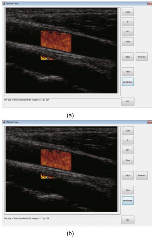
**Fig. 7** GUIs using the proposed demodulation method (a) and the conventional quadrature demodulation method (b). The color flow map reveals the velocity distribution in a healthy common carotid artery. References to color refer to the online version of this figure
