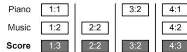
Fig. 2 An example showing the index traversal procedure of DAAT with two posting lists of the query terms ‘piano’ and ‘music’. The solid line separates different iterations of the procedure from left to right, and the scoring operation scans from top to bottom in each iteration to sum up all of the term frequencies f_{t,d} . The full result score of a document can be obtained when both ‘piano’ and ‘music’ are considered in parallel. Reprinted from Jiang and Yang (2015), Copyright 2015, with permission from Springer
