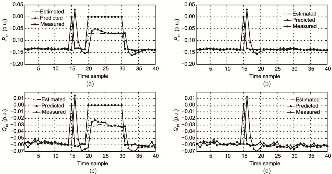
**Fig. 3** Active and reactive power injection at bus 13: (a)  $P_{13}$  before correction; (b)  $P_{13}$  after correction; (c)  $Q_{13}$  before correction; (d)  $Q_{13}$  after correction
