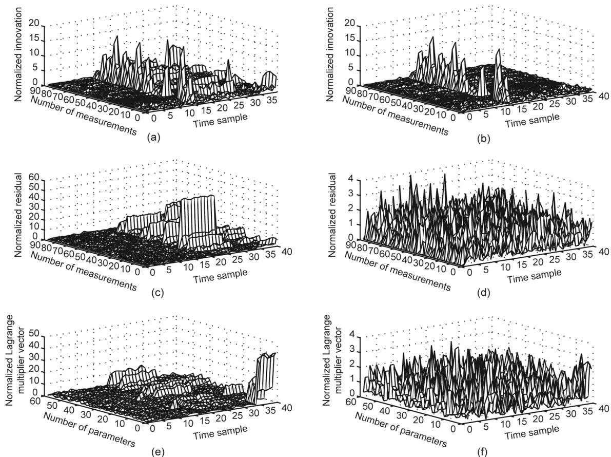
**Fig. 4 Variations in normalized vectors: (a)  $v_{k+1}$  before correction; (b)  $v_{k+1}$  after correction; (c)  $r_{k+1}$  before correction; (d)  $r_{k+1}$  after correction; (e)  $\lambda_{k+1}$  before correction; (f)  $\lambda_{k+1}$  after correction**
