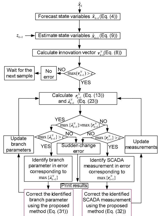
Fig. 1 Flowchart of the proposed algorithm (SCADA: supervisory control and data acquisition)
