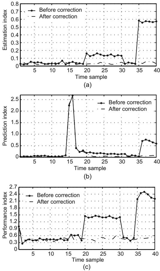
**Fig. 2** Variation in evaluation indexes on the IEEE 14-bus test system: (a) estimation index; (b) prediction index; (c) performance index
