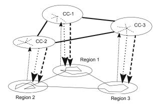
Fig. 4 ECPS of the IEEE 39-bus system. Dashed lines: channel 1 (e.g., C-(1)); dotted lines: channel 2 (e.g., C-(2)); bold dashed lines: channel 3 (e.g., C-(3)). Arrows represent the directions of information flows
