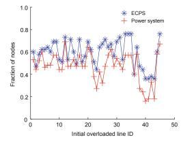
Fig. 8 The scale of cascading failures in the IEEE 39-bus system
