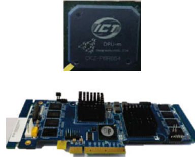
Fig. 4 High-throughput many-core processor DPU chip
