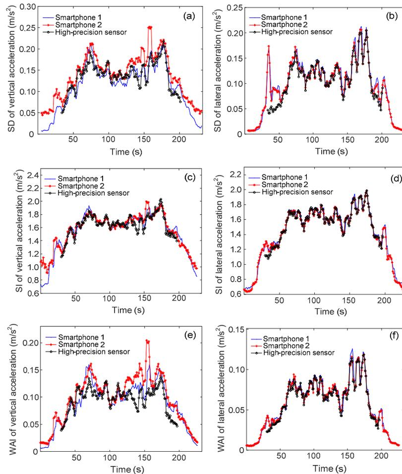
**Fig. 12** Comparison of evaluation indexes with 5-s moving window: SD (a), SI (c), and WAI (e) of the vertical acceleration, and SD (b), SI (d), and WAI (f) of the lateral acceleration
