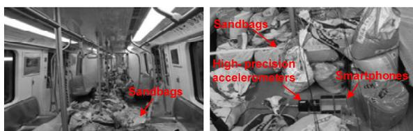
Fig. 4 Field test setup
