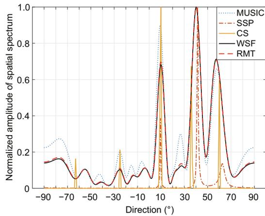
Fig. 2 Normalized amplitude of spatial spectrum versus the search direction ranging from  $-90^\circ$  to  $90^\circ$  (SNR:  $-8$  dB; number of snapshots: 10)
