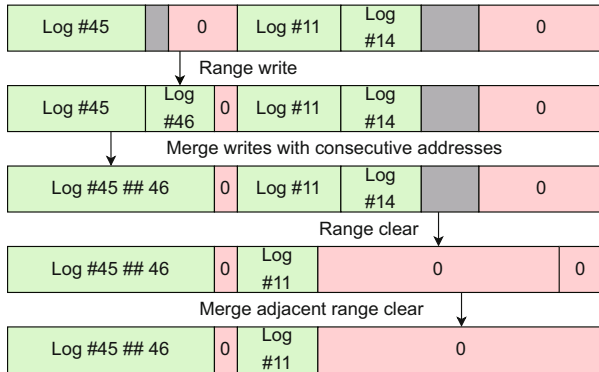
Fig. 7 Merge algorithm for modifications to a data block
