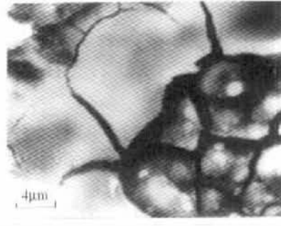
Fig. 6 SEM of worn boronised sample in the initial stage with \text{Al}_2\text{O}_3 at 90^\circ impacting angle.
