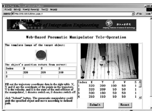
Fig.6 Define the movement of the manipulator
