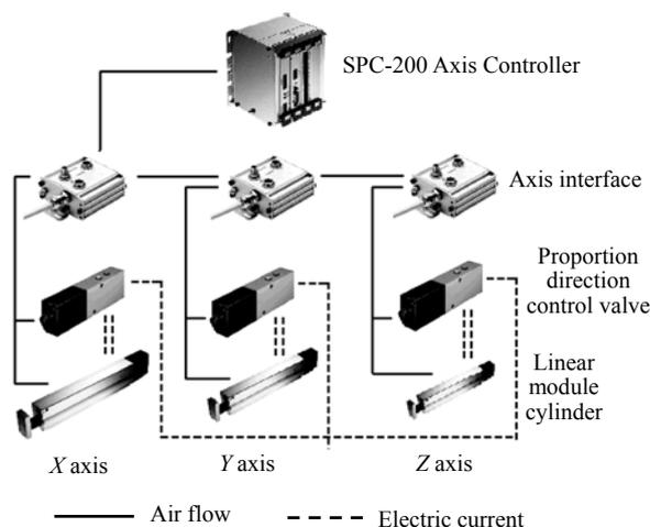
**Fig.2 Structure of the SPC-200 electro-pneumatic proportional/servo control system**
