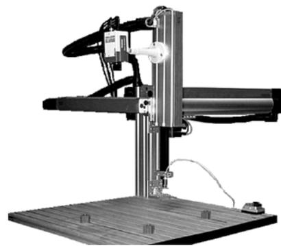
**Fig.1 Three-degrees-of-freedom pneumatic manipulator**
